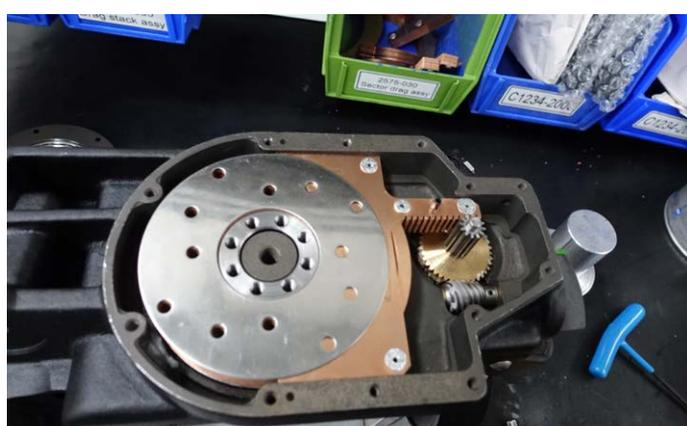
13. Place drag assembly into base casting.
