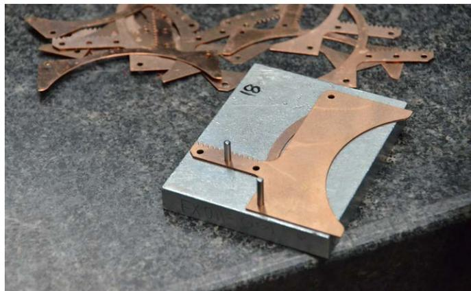
9. Stack one set of copper plates together with spacers on a jig.
